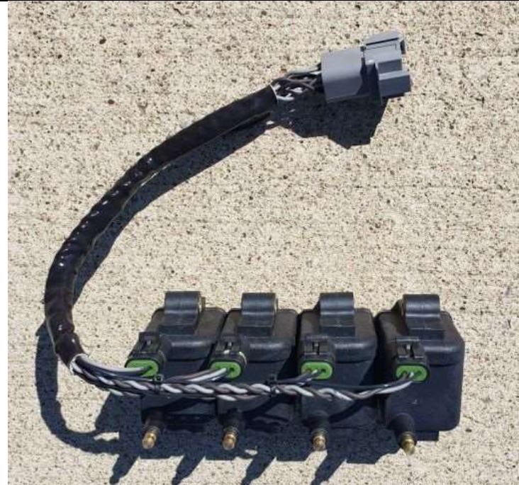
Pro-600 Coil Bank with custom harness
